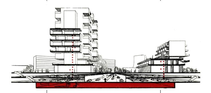
Figure 4: Section of a typical neighbourhood center, service distribution in color.
